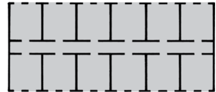
HIGH-RISE BEARING WALL CONFIGURATION (shown in plan)
