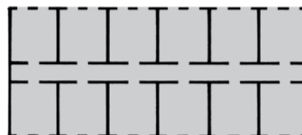
HIGH-RISE BEARING WALL CONFIGURATION (shown in plan)
