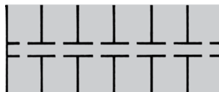
LOW-RISE BEARING WALL CONFIGURATION (shown in plan)
